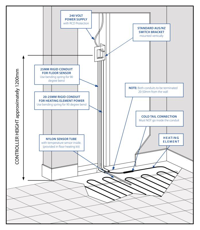
For tile over heating element installations, the floor may need to be chased to allow the sensor tube and cold tail connection to sit low enough to be tiled over.
